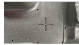
At left, a closeup of the "plus" registration mark engraved on every thermoformed part that enters the vision guided trim stations at all Prent facilities.
